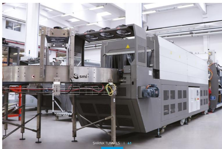
Having a tunnel powered by natural gas instead of electricity is advantageous, especially where natural gas is available at affordable prices. In fact, comparative tests have shown that, where the conditions exist, a methane-fueled shrink tunnel allows for savings of up to 40% on energy costs compared to traditional power supply. 🍗
