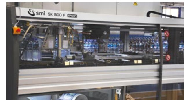
For the bottling and packaging of the natural spring water under the Lejdar brand, Tousnina Sarl turned to the experience of SMI, who supplied a complete turnkey line, supporting the customer during design, construction and installation of the 20,000 bottles/hour plant. Apart from the complete line, the Algerian company also bought an EBS 4 ERGON, to integrate in a pre-existing 8,400 bottles/hour line for the production of 0.33 L, 1 L and 2 L PET bottles for bottling carbonated beverages.
