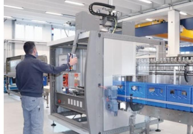
operation of the two production lines when the packing of PET bottles is carried out in shrink film bundles.
