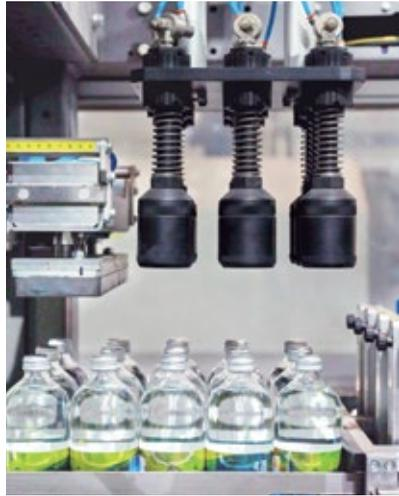
➤ **ACP 20 S ERGON CASE PACKER with separator insertion device**
