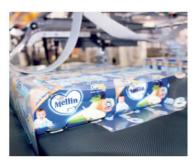
The process of packing in film is extremely fluid: on the machine infeed conveyor, equipped with low-friction chains made of thermoplastic material, loose containers are clustered in the desired format by a pneumatic device and electronically synchronised separating bars before accessing the film wrapping section and the shrink tunnel.
