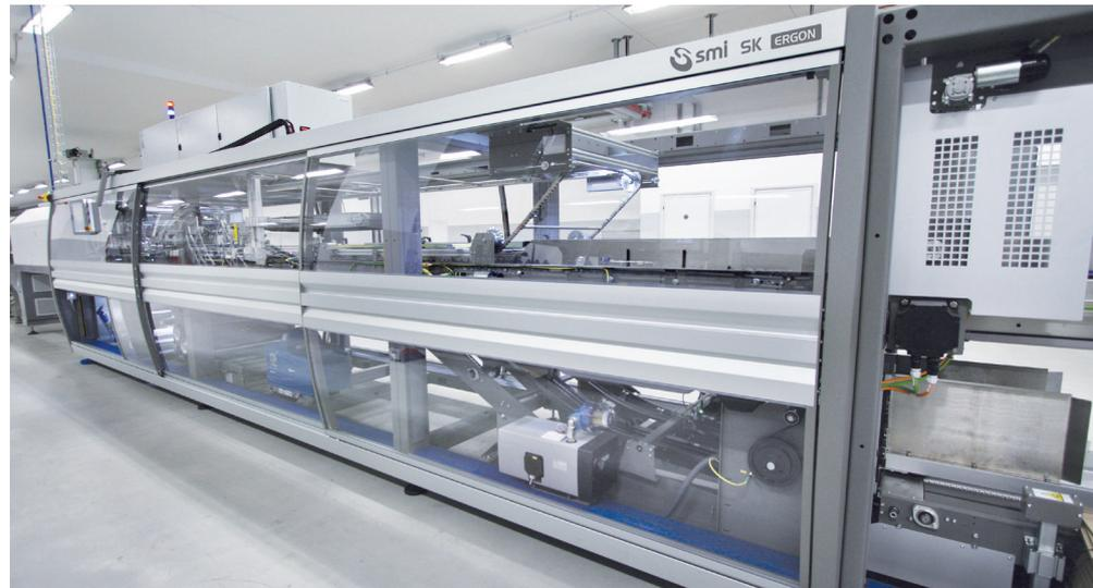
generated by the shrinking process, SMI tunnels are capable of handling in an efficient and homogeneous way the distribution of hot air flows over the whole area of the pack.
