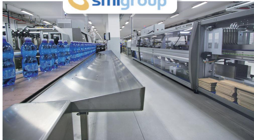
The machine model exhibited at Brau Beviale will be equipped with a device to handle products in dual lane, that permits to wrap two packages of 6 cans simultaneously (3x2 film only format) and to achieve in this way a maximum output capacity of 160 packs/minute (80 packs/minute on each lane).
