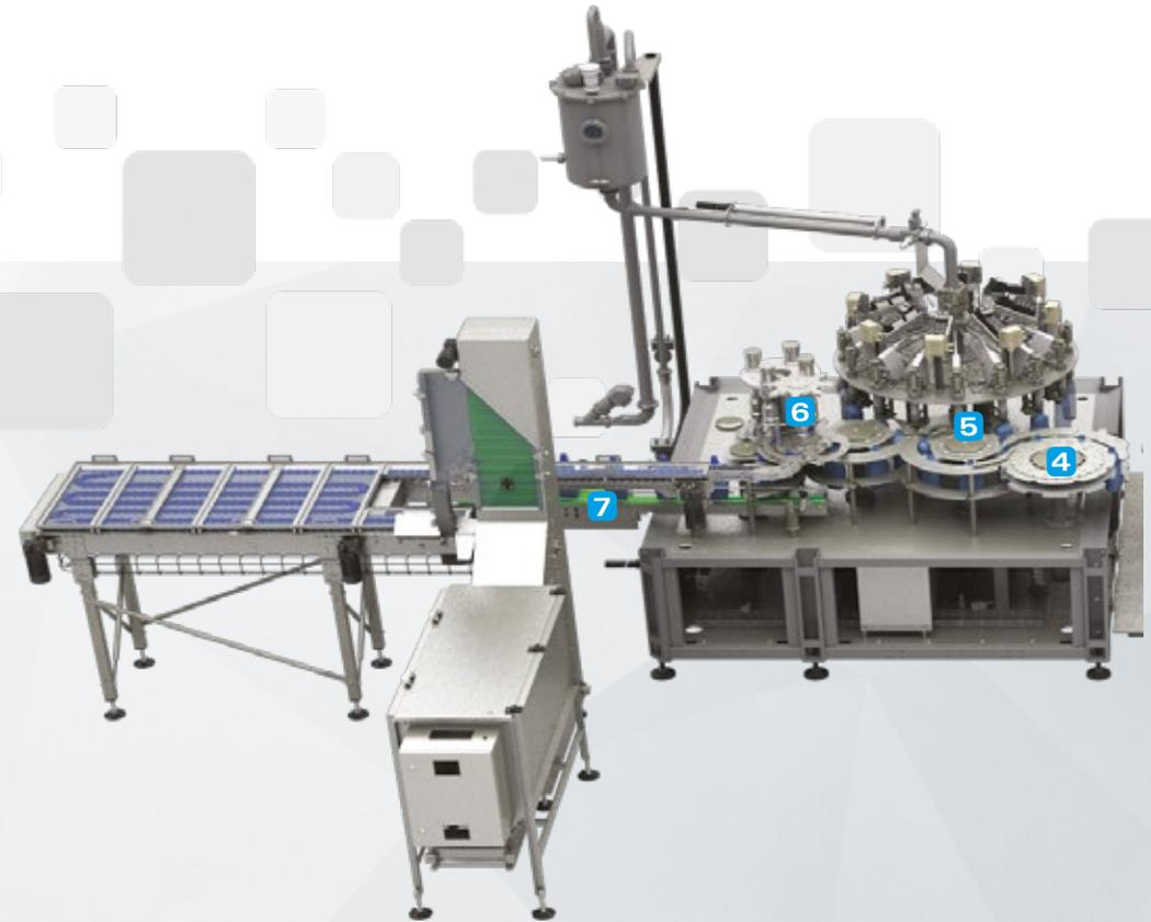
sniff phase starts: a specific channel conveys the pressure left in the bottle to a dedicated manifold that discharges outside the filling section. At this stage the bottle is transferred to the capper.
