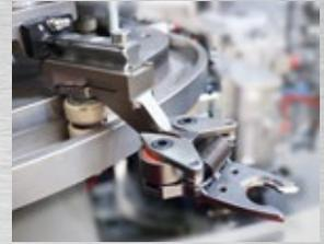
• The grippers boast a sensor-equipped clutch, ensuring that each gripper always keeps the phase position.
