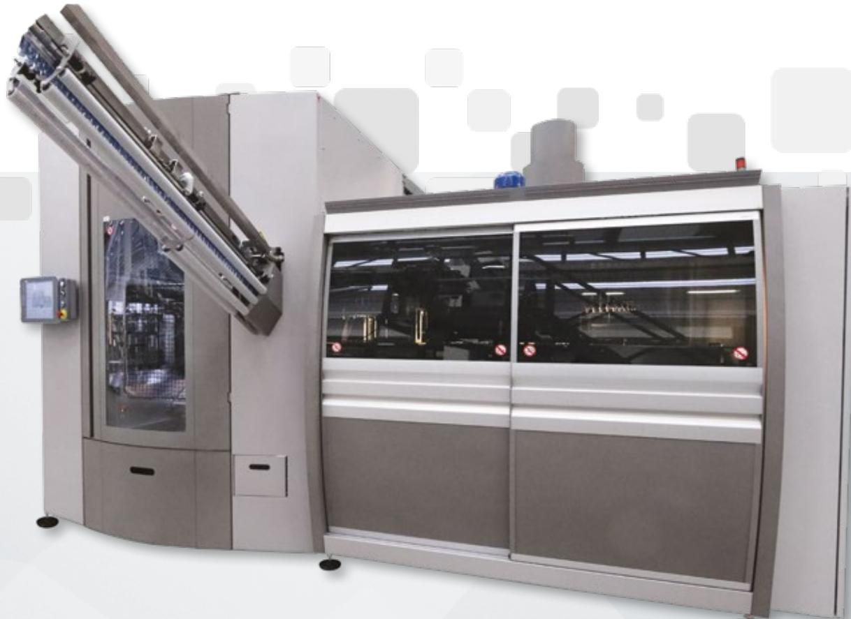
The EBS E ERGON project is based upon all-electronic processes which allow to get rid of the whole of mechanical movements and related cams and ultimately make the blower a cam-less machine.
