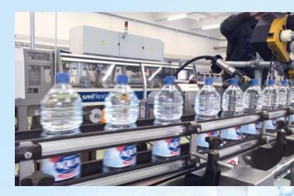
he 12,000 bottles per hour bottling line installed in the plant in Zhdanovichi makes use of a latest generation automation and control system called VaryLine System® that, together with the use of sophisticated sensors, allows you to maintain high levels of operational efficiency throughout the production cycle, thus reducing costs and energy consumption.
