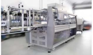
To optimise the secondary packaging process of the huge variety of "Le Conserve della Nonna" brand products, the Fini Group turned to SMI for the installation of an automatic shrinkwrapper from the CSK ERGON series, which stands out for its advanced automation and flexibility of use, low energy consumption and respect for the environment.
