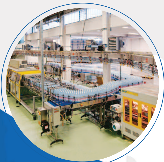
Production line with SMI machines (shrink wrappers and conveyors)
