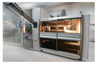
The EBS Ergon series dispenses with cams to minimise energy consumption while maximising performance and ease of use.
