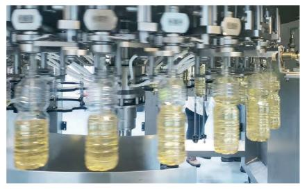
The wide range of solutions offered by SMI also include that with the weight filling system.
