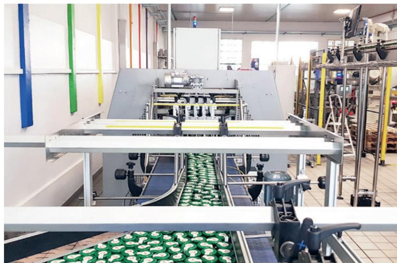
LSK 40T shrink wrapper is the best solution for packing in tray+film or pad+film the wide range of jars produced by Cereal Terra.
