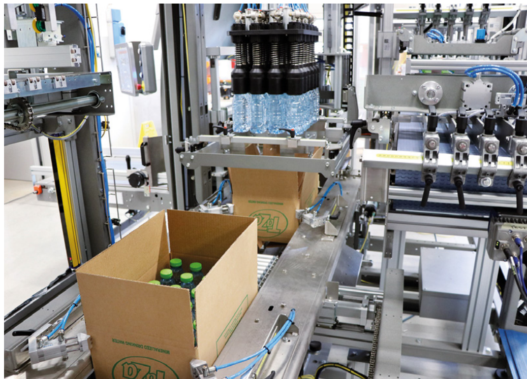
Monobloc case packer with pick & place system for RSC boxes at the All4pack 2022 show (SMI)
