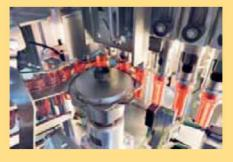
9,200 bph, the EBS K models are available in 2, 3 and 4-cavity versions, and offer all the advantages of rotary technology in a "speed" range traditionally controlled by linear stretch-blow moulders, states the company.
