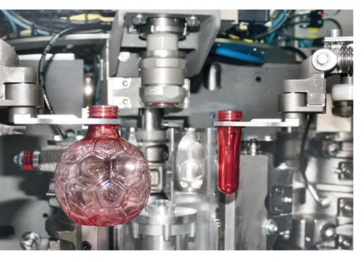
sures precise control of the path of the stretch rod, significant energy savings and reduced mechanical interventions;
