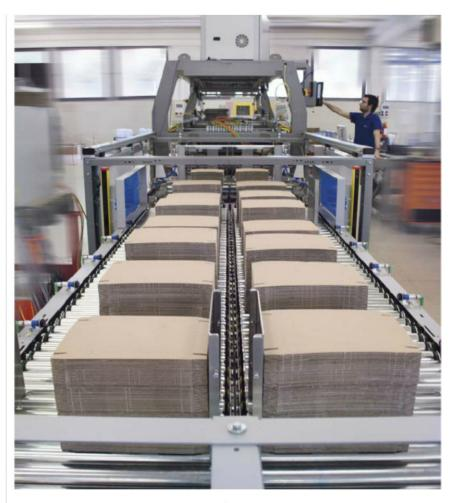
the wrap-around case packers of the WP series and the heat-shrink-wrappers of the SK series) which features considerable advantages from an operating and functional point of view. With Easy-Load the operator can easily load cardboard blanks - stacked horizontally in uniform groups - because the feeding belt of the magazine is posi-
